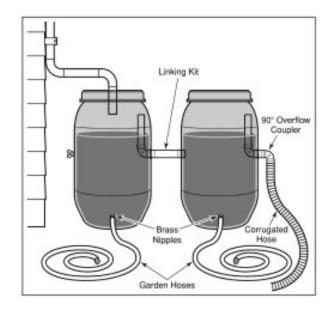
1. **Rain Barrels**. They are great for collecting rain and runoff from your home's downspouts, providing naturally soft water loved by plants. You can place the barrel under the down spout as shown in the figure or you can use an automatic diverter to direct the rain back into the downspout once the barrel is full.
